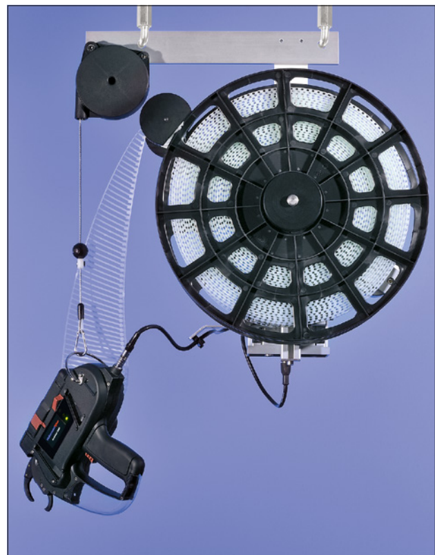
Overhead Suspender, reel with cable ties and Autotool 2000.
